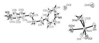
Figure 1. The building-block unit present in crystalline 1. Thermal ellipsoids are drawn at the 50% probability level. Selected bond lengths [Å] and angles [°]: Mo(1)-O(2) 1.671(3), Mo(1)-O(1) 1.683(3), Mo(1)-O(1W) 2.217(3), Mo(1)-O(2W) 2.244(3), Mo(1)-Cl(1) 2.3739(13), Mo(1)-Cl(2) 2.3754(15), O(2)-Mo(1)-O(1) 105.12(16), O(1W)-Mo(1)-O(2W) 75.33(12), Cl(1)-Mo(1)-Cl(2) 162.13(6).
